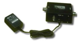
Frequency Range: 20 MHz – 4 GHz Gain (typical): 26 dB Gain (minimum): 22 dB Flatness: +/- 5 dB Noise Figure: 4.5 dB Output Power @ 1 dB compression + 15 dBm Input VSWR (typical): Less than 1.7:1 Output VSWR (typical): Less than 2.0:1 Connector: N-Type, female
