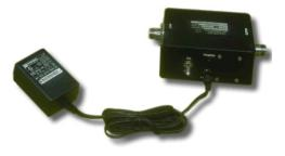
Frequency Range: 5 KHz – 300 MHz Gain (typical): 32 dB Gain (minimum): 28 dB Flatness: +/- 1 dB Noise Figure: 2.1 dB Input VSWR (typical): Less than 1.5:1 Output VSWR (typical): Less than 1.5:1 Connector: N-Type, female
