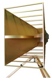
Frequency Range: 170 MHz - 3 GHz Antenna Factor (1 Meter): 11 to 33 Gain (dBi): 0 to 10.9 Maximum Continuous Power: 800 Watts Impedance: 50  $\Omega$ Max Radiated Field: 200 V/m 500 V/m (with Optional 7/16 DIN female connector) Connector: N-Type, female
