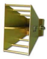
Frequency Range: 700 MHz – 18 GHz Antenna Factor (1 Meter): 22 to 44 Gain (dBi): 1.4 to 15 Maximum Continuous Power: 300 Watts Max Radiated Field: 200 V/m 3 dB Beamwidth (E-Field): 48° (average) 3 dB Beamwidth (H-Field): 30° (average) Impedance: 50  $\Omega$ Average VSWR: < 2:1 (3.5:1 max) Connector: N-Type, female Mounting Base:  $\frac{1}{4}$  - 20 Thread, female
